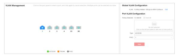
**Figure 4-11 Configure Port VLAN**
