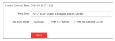
Figure 5-3 Configure Time with Hik-Connect Server
